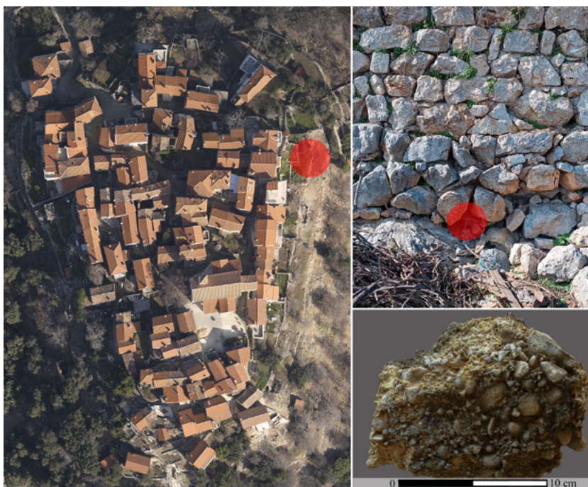
Figure 6: Aerial Image of Beli, Showing the Sampling Point for The Mortar Dating (Red Dot), a Relevant Section of the City Wall, and the Mortar Sample in Detail (project-owned aerial image, elaborated by Nives Doneus, 2025)
